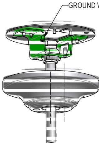
**NOTE:** THIS FIXTURE MUST BE MOUNTED INDEPENDENTLY OF A JUNCTION BOX
